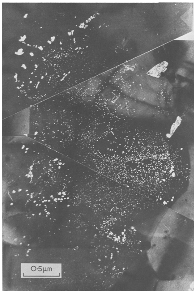
Figure 1 TEM dark field micrograph showing the distribution of \text{Al}_3\text{Zr} particles.
